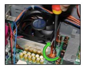
TIP: Follow the sequence shown: half-tighten the screw on one corner of the heatsink and fan, then the next screw on the other corner and so on, making a cross pattern. Repeat until all four screws are tightened properly.
